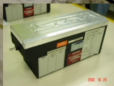
Increased Capacity Battery (ICB) for EMU Silver-Zinc (Ag/Zn)
