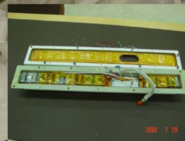
Simplified Aid For EVA Rescue (SAFER) Battery Lithium Manganese Dioxide (Li-MnO 2 )
