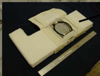
Rechargeable EVA Battery Assembly (REBA) Nickel Metal Hydride (NiMH)
